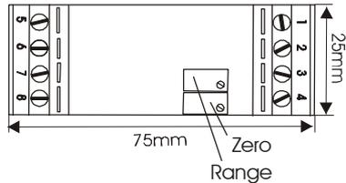
To open the clear view cover this must be carefully pressed inwards on the narrow sides and lifted off. The location of the potentiometers can be seen in the adjacent figure. The potentiometers are protected against inadvertent adjustments. The null point potentiometer can be adjusted to make small corrections. The range potentiometer should be adjusted as little as possible.
