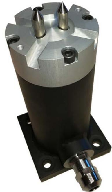
The probe tips in diameter 7,0 mm are biased by springs and by the hydraulic or pneumatic forward stroke with a spring force of about 28 N against the surface to be measured pressed. The measured value is available immediately after touching the probe tips to the metal surface. The spring path of the probes may be up to 20 mm.
